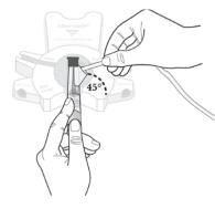
Insert the PIN connector at a 45 degree angle into the opening of the organizer clip. Press down on the PIN connector to ensure a snug fit in the organizer clip.
